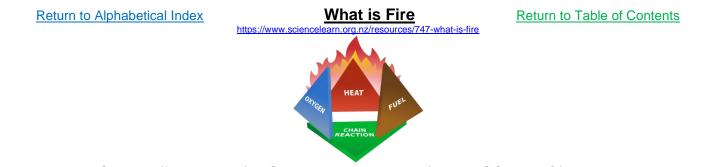
Fuel + Oxygen (from the air) = Combustion Products (mainly  $CO_2 + H_2O$ ) + Heat Energy <u>Fire Triangle</u> - Illustrates the three elements a fire needs to ignite: Heat, Fuel and Oxygen. For fire to start, or have combustion, the fuel must be heated to ignition temperature that varies by the fuel.
